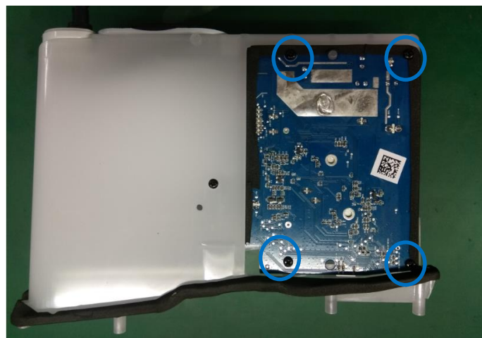
5.3 Unscrew the 4 screws, remove the main board.
