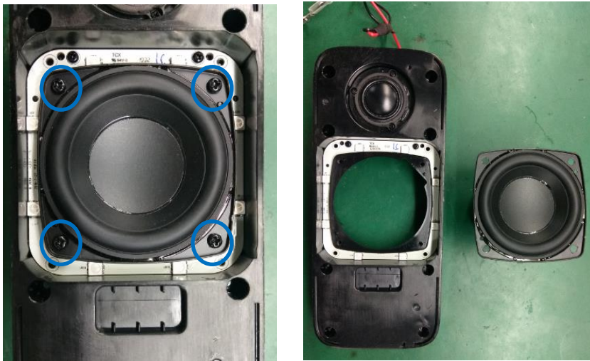
4.4 Unscrew the 4 screws, remove the woofer .
