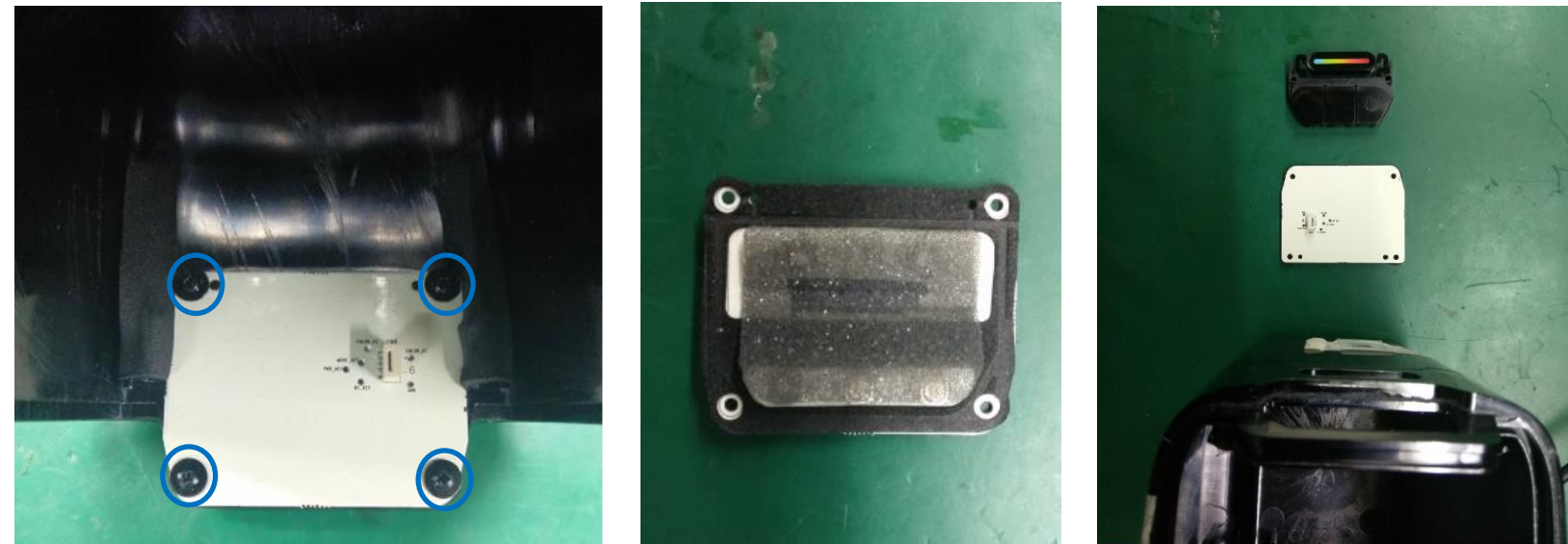
5.2 Unscrew the 4 screws, remove Mechanical key circuit board and mechanical key.
